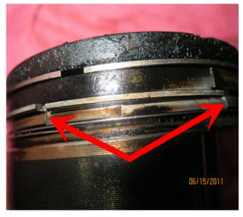
If cracked piston ring lands are found, then inspect the cylinder head to determine first or second design. See photos below.
