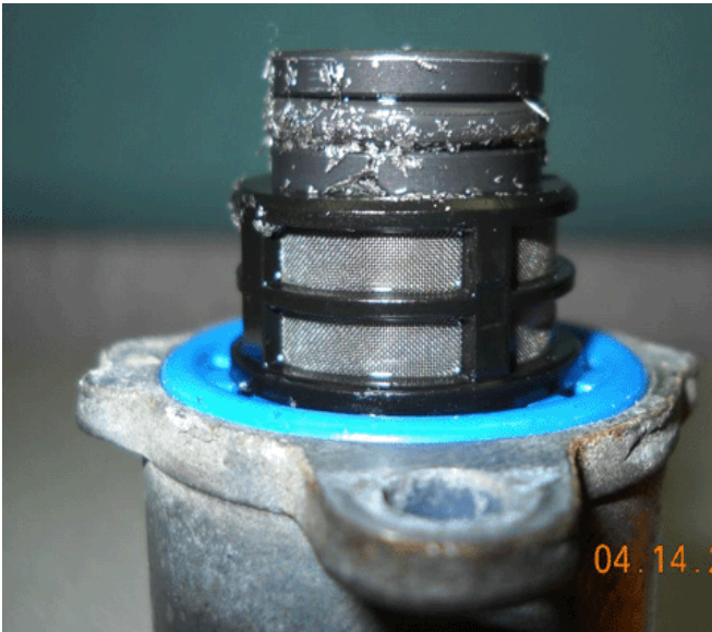
Contaminated Fuel Pressure Regulator 1 (View B)
