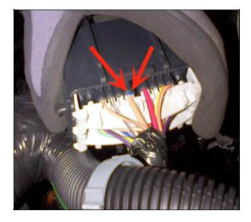
Inspect connector X109 before disconnection. Terminal A5, motor circuit (1552) is visibly backed out in the image above.
