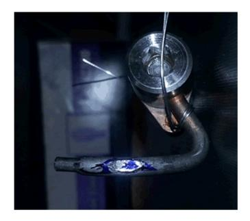
If contact is noted the dealer needs to call PQC for a replacement engine. (PER PIP5114) Pictures of normal crankshaft marking that are not caused by the oil squirter making contact.
