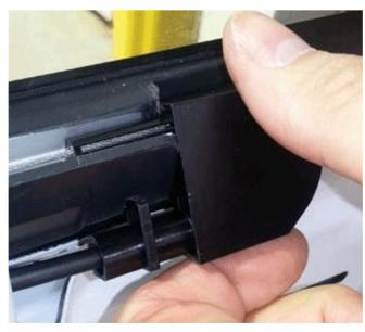
If the cable pulley cover completely disengages, the pulley can come off and cause the cable to bind, see photo below.
