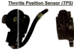
**Functional Description**: This sensor detects the throttle valve opening angle.
