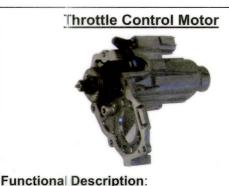
Adjusts the throttle valve opening angle in accordance with signals from the ECM.
