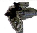
Functional Description: Adjusts the throttle valve opening angle in accordance with signals from the ECM.
