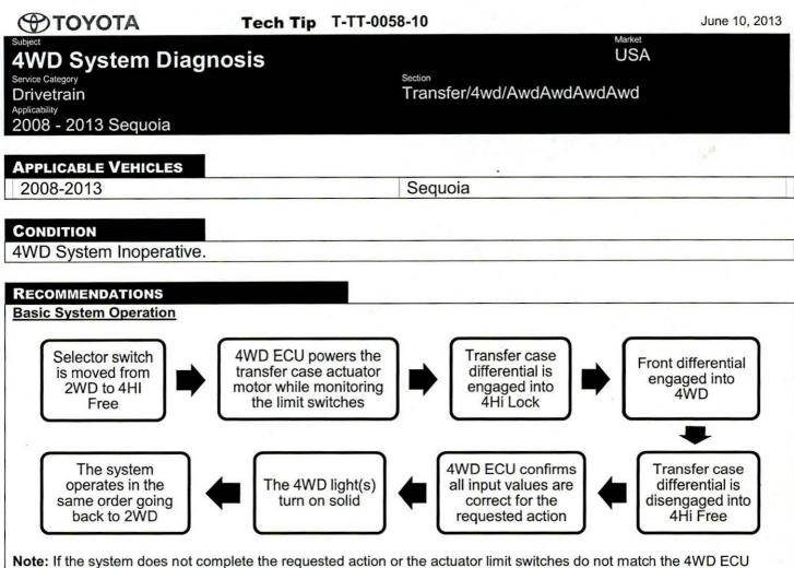
**Note:** If the system does not complete the requested action or the actuator limit switches do not match the 4WD ECU desired position, the 4WD light(s) will flash indicating a problem. Additionally if the system is unsure of its position, it may stop operating and not move in or out of its current position.
