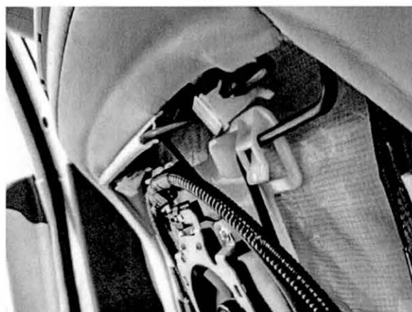
View of the clip once it has been successfully detached from the seatback cover
