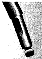
Bent or dented shock
