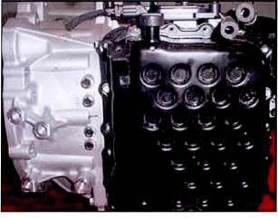
Filling and checking of fluid level is done through valve body side cover
