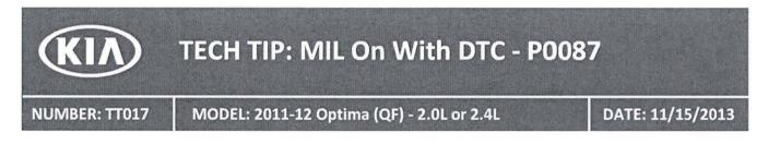
Symptom: Low power and MIL on with DTC - P0087 (Fuel Rail/System Pressure - Too Low)
