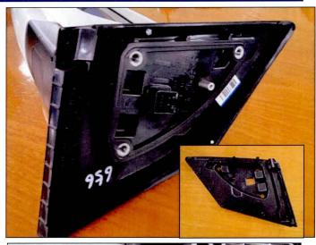
6. Remove base cover cap as shown in the picture.
