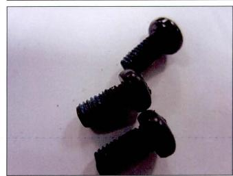
9. Apply Loctite\* to the screw as in the photo.
