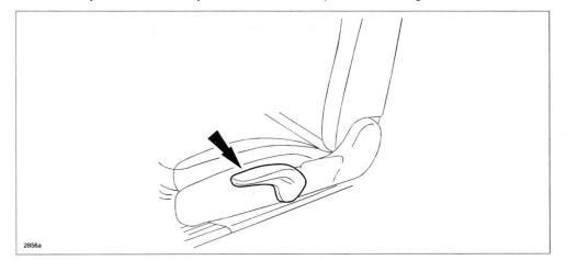
This may be caused by a broken front seat side cover that interferes with the operation of the seat lifter mechanism. The cover may have been previously broken by an outside impact.
