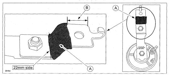
Reinstall the theft-deterrent horn with the installation bolt.
