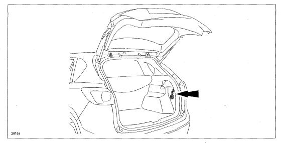
An EPT sealer has been attached to the theft deterrent horn during mass-production to eliminate the noise. Customers having this concern should have their vehicle repaired using the following repair procedure.
