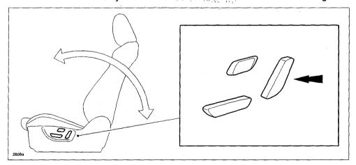
The configuration of the recliner switch knob has been changed to eliminate this concern. Customers having this concern should have their vehicle repaired using the following repair procedure.
