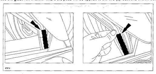
5. Apply an adhesion promoter (one that is suitable for use on plastic) to the two (2) locations where the pads will be attached.
