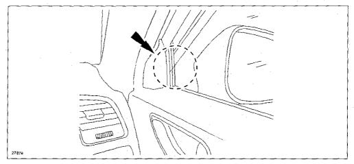
The rattle noise may be caused by insufficient glass run channel holding force. To eliminate this concern, the shape of glass run channel has been changed in order to increase the holding force.
