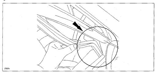
4. Degrease the glass run channel where the pads will be applied to the two (2) locations shown below.
