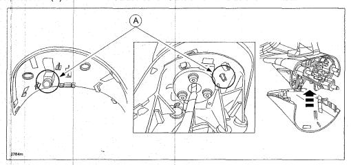
15. Confirm the harness length from the mirror base to the end of the connector is 340mm +- 10mm (A).
