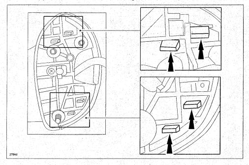
7. If the connection is disconnected, remove the cover by pulling it in the direction of the arrow shown below.
