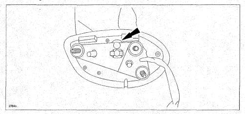
17. Remove the old EPT sealer from the harness and wrap a new one (included in the base cover set) in the same position (A), 140mm from the end of the connector.
