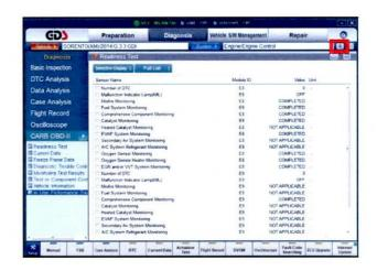
9. Select "Entire GDS Area" and click "Send to file." The GDS will set up a designation folder and file name to save the captured data. Please change the file name to include the model/engine, the last 6 digits of the VIN and the date (mmddyyyy). Before saving, write down the file name and designation folder for further reference.
