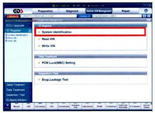
5b. Do a screen capture of "Calibration ID" or "ROM ID" number for later form entry. Select "Entire GDS Area" and click "Send to file". The GDS will set up a designation folder and file name to save the captured data. Please change the file name to include the model/engine, the last 6 digits of the VIN and the date (mmddyyyy). Before saving, write down the file name and designation folder for further reference.
