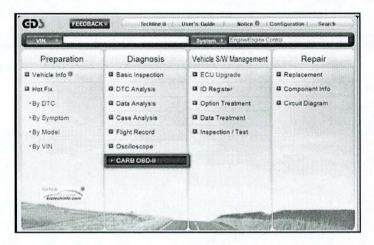
Click on "IN-USE Performance Tracking" found in the CARB OBD-II list at the bottom left of the screen. Then click the "Expand" button at the top right corner of "IN-USE Performance Tracking" window.
