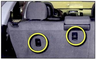
Remove the j-hook and hog retaining ring on the bottom of the LH seatback. Use pliers to remove the hog ring.
