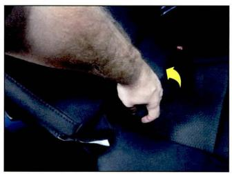
8. Make sure the cable guides are properly seated in the retaining brackets on the seatback frame. Also, inspect the cables for damage. If a cable is damaged, replace it.
