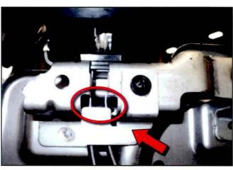
12. Remove two screws securing the cover on the outboard seatback recliner mechanism.
