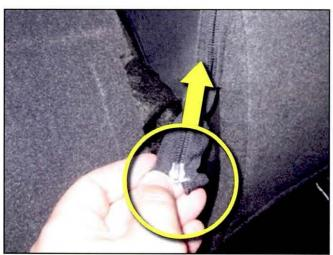
5. Locate and unzip the RH zipper tucked underneath the seatback covering.
