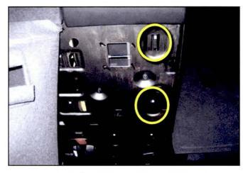
8. Remove the j-hook securing the bottom seat cushion covering.
