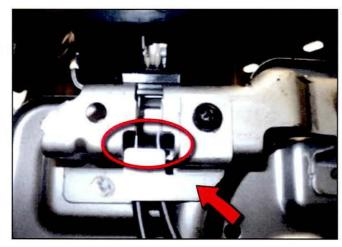
Remove two screws securing the cover on the inboard seatback reclining mechanism.
