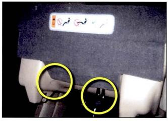
4. Locate and unzip the LH zipper tucked underneath the seatback covering.
