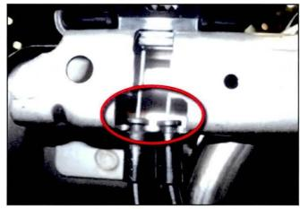
11. On vehicles produced on or after September 15, 2011, remove the bracket to ensure the cable guides are properly seated in the retaining brackets on the seatback frame. Also, inspect the cables for any sign of damage. If a cable is damaged, replace it.
