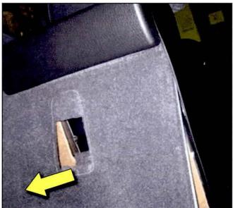
Lift the seatback trim material and remove the 8 clips retaining the seatback board. Do not pry against the seat back board while removing the retaining clips.
