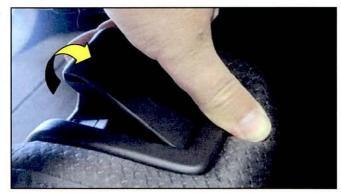
Remove both child seat anchor bezels using a non-marring trim removal tool (such as Snap-on® Part Number PBN5 or equivalent).
