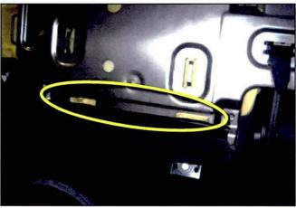
Lift seatback cushion to expose the reclining handle, cables and reclining mechanism.
