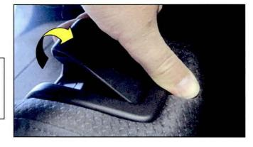
To correct the concern on the RH side (40%) of the 2nd row seat, replace both inboard and outboard reclining mechanisms. Refer to KGIS > Body > Seat & Power Seat > Rear Seat > Repair Procedures, for specific repair procedures.
