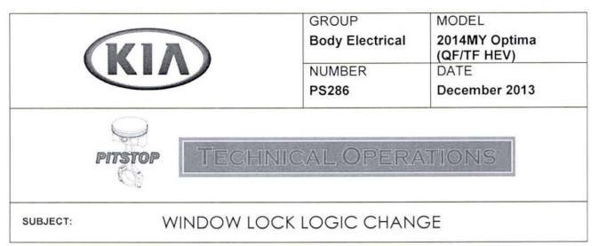
To improve feature usability, and customer satisfaction, a modification has been implemented to the logic of the power window lock feature on the 2014MY Optima (QF/TF HEV). Activation of the window lock feature will no longer apply to the front passenger window, only the rear driver and passenger side windows. Additionally, all windows can now be controlled from the master switch, regardless of the lock switch position.
