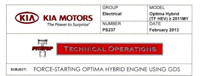
If you encounter an Optima Hybrid with a no-start condition, check if the "READY" lamp is flashing in the cluster and verify the hybrid battery State of Charge (SOC) ranges from 15% to 20%. If these conditions are present, a technician may use GDS to "force start" the engine and resolve the concern.
