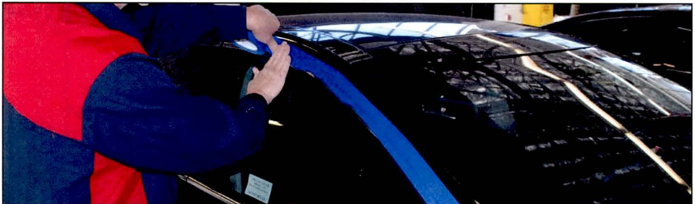
By taping off sections at a time, this aids in narrowing down the area of the suspected noise.
