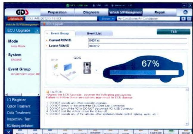
12. Follow the guidelines displayed on the screen during upgrade procedure and make sure to cycle the ignition **OFF** → **ON** one (1) time.
