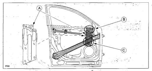
11. While holding the power door mirror, temporarily place the reinforcement with the three (3) power door mirror bolts through the holes in the reinforcement, then tighten the bolts.
