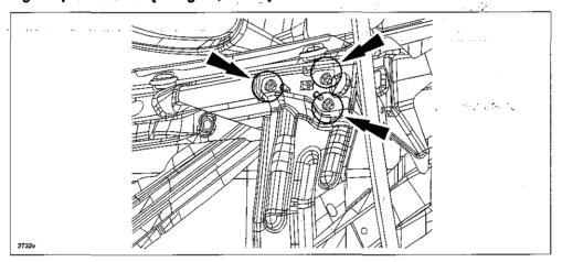
12. Place the two (2) brackets (A) (upper and lower) in the back of the reinforcement and pass the stud bolts through the holes in the reinforcement.
