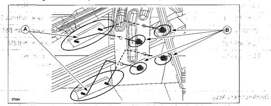
13. Tighten the four (4) nuts (B) to secure the reinforcement onto the side impact bar-lower. Tightening Torque: 15 ft. lbf. {2.1 kgf-m, 20 Nm}
