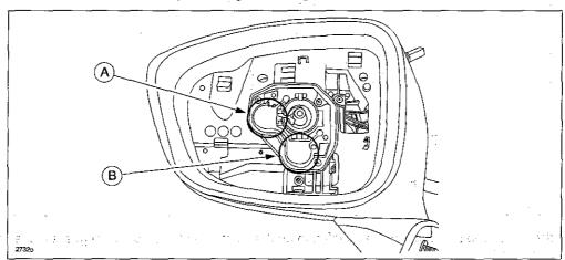
3. Place the mirror glass on the mirror base aligning the location of the center pivot (A).
