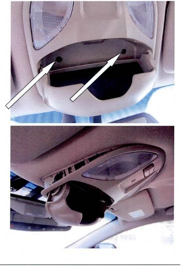
4. Separate the overhead console from the headliner by pulling the sunglass holder case downward.
