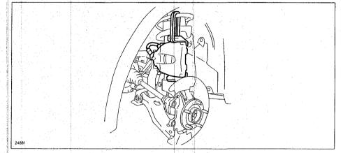
13. Remove the front lower arm ball joint bolt (A) and nut (B). Then separate the lower control arm from the knuckle.
