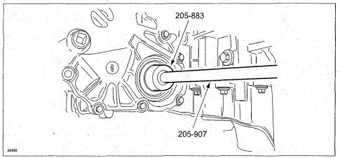
21. Use SST part number 205-907, part number 308-221, and part number 308-431 to install the new oil seal.
