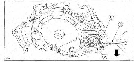
20. Use SST part number 205-907 and part number 205-883 to install the new transfer dust seal.
