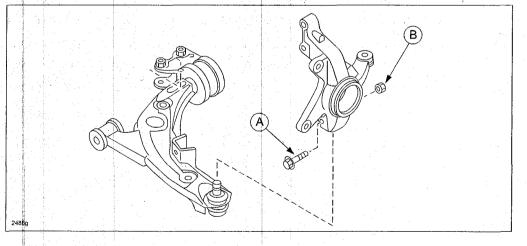
14. Pull the knuckle outward, rotate it toward the rear of the vehicle, and secure it.
