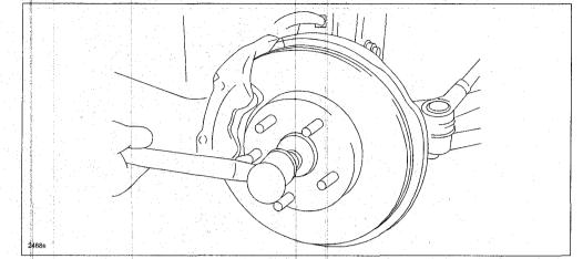
12. Remove the brake caliper component from the steering knuckle and suspend it out of the way using a cable.
