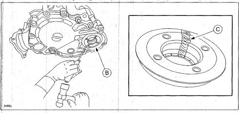
18. Use SST part number 49S2-31-660 to remove the transfer dust seal.
