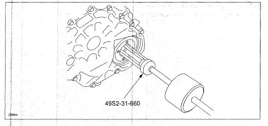
**NOTE:** Do not reuse the removed deflector (B). If the deflector is difficult to remove using SST 49S2-31-660, break the deflector by using a flat-blade screw driver for hammering (C).
