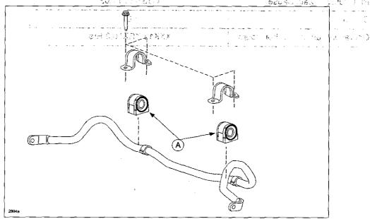
NOTE: To prevent noise from occurring, never apply any type of grease or lubrication to the front or rear stabilizer bushings.
