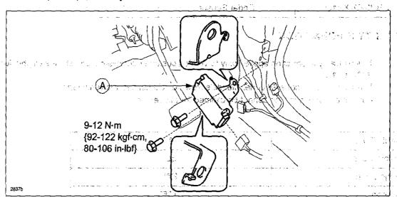
· RADAR SENSOR REMOVAL/INSTALLATION [MAZDA RADAR CRUISE CONTROL (MRCC) SYSTEM]
