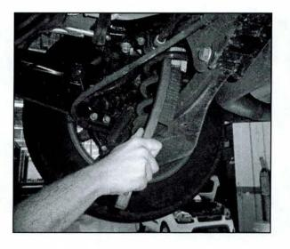
Spray cavity wax into all holes from the underside of the rear lower control arms, as shown.
