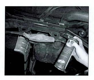
Apply underbody coating onto all surfaces of the cross member, as shown. Avoid over-spraying other vehicle components.
