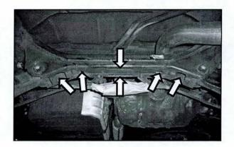
Spray cavity wax through the holes in the underside of the cross member, as shown.
