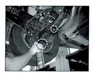
Spray cavity wax, at two separate locations, from the top of the rear lower control arms, as shown.
