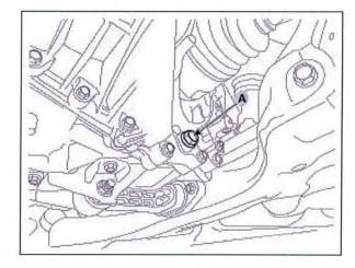
2. Install the drain plug.
