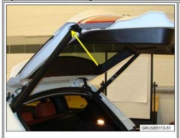
1. Locate the hex bolt securing the tailgate strut holder. Shown is the driver's side tailgate strut. Support the tailgate with a suitable device. Using Repair Instruction 51 24 350, remove the tailgate strut/spindle drive.
