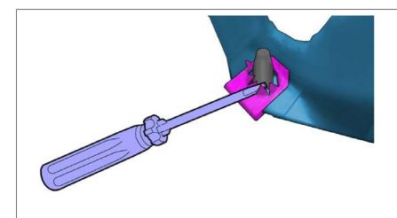
Note! Carefully bend the clips loose without damaging the clip mountings in the bottom of the tank.
