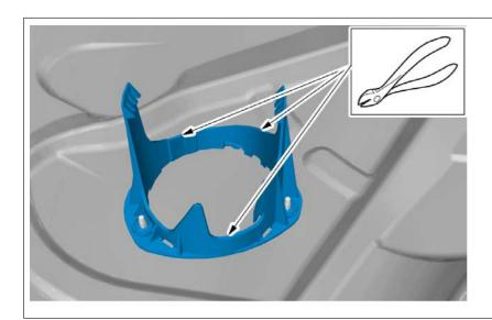
Note! Cut the holder into three pieces to access the clip.
