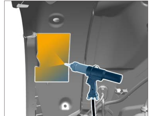
Applying underbody protection
