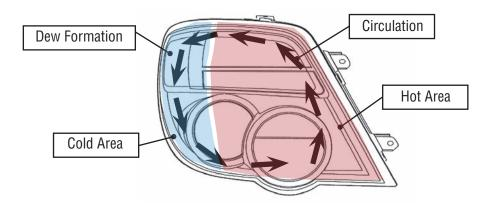
2) If an already warm lamp lens gets cooled down rapidly (e.g. when water is applied to the lens during vehicle washing), a sudden temperature change can occur resulting in the development of condensation.
