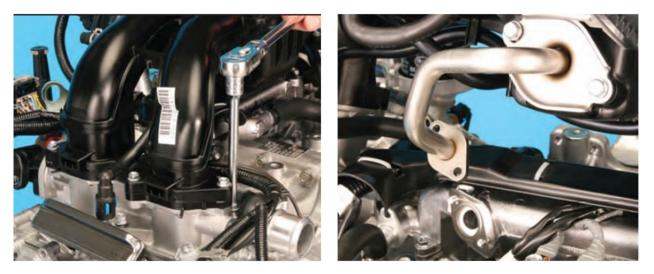
• There is no need to remove the oil dipstick tube or the original oil filter from the front chain cover. While the cover is removed, store it face (front side) down to minimize the chances of damaging the machined sealing surface on the block / head side. Also, don't use it as a tray to store other removed parts. This will help to reduce the chances of contamination entering the various oil passages throughout the front cover.
