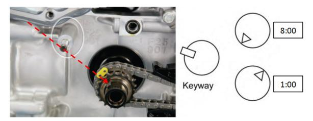
Align the indicator links to the timing marks found on the outside of the sprocket assemblies as shown in the photos below (Exhaust sprocket face images will vary with / without exhaust VVT).
