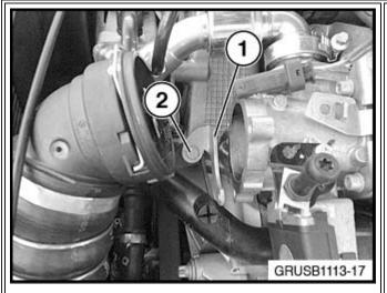
Install bracket P/N 13 54 8 576 446 (1) to the cylinder head using the bolt P/N 07 11 9 904 527 (2). Leave this bolt finger tight until after the throttle valve is reinstalled.
