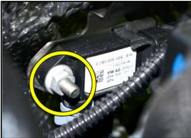
⇐ Remove the differential pressure sensor mounting nut <circle>.
