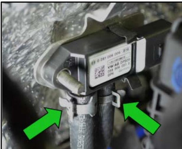
⇐ Reposition the spring clamps on both of the particulate filter hoses to allow removal of the hoses from the differential pressure sensor <arrows>.
