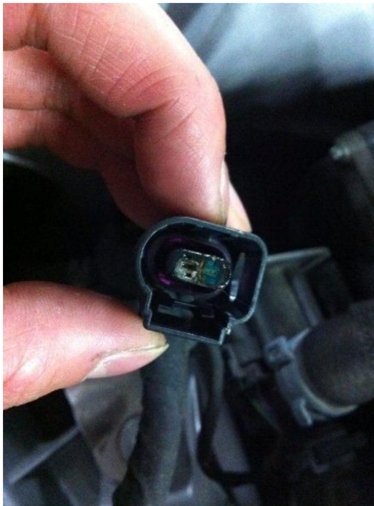
Figure 2. Corrosion formation on the connector pins.
