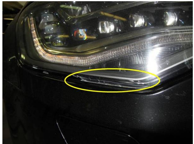
Figure 3. Lower headlight lens cracking.
