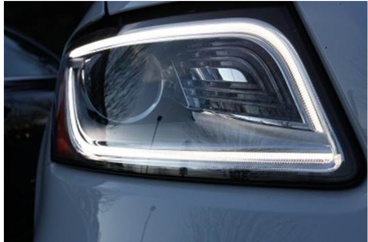
Figure 1. Upper and Lower light pipe illuminated.
