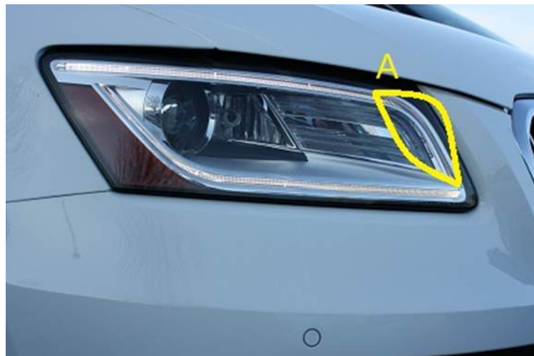
Figure 4. Upper light pipe perceived defect (A).
