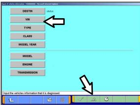
g. If the VIN or vehicle description displayed does not match the vehicle you are working on, click on the eraser icon at the bottom of the page to erase vehicle data.
