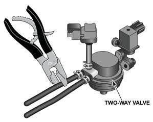
Disconnect the purge hose from the canister and connect a vacuum pump to the canister fitting.
