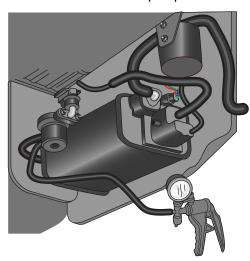
Enter the HDS PGM-FI menu, and select INSPECTION> EVAP TEST> SINGLE SOLENOID> BYPASS SOLENOID. Click the green check box to turn ON the BPS valve.
