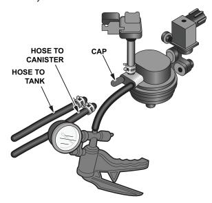
Watch the FTP sensor value on the HDS, gently apply vacuum until the value reads approximately 1.50 V (it takes very little vacuum to reach this value).
