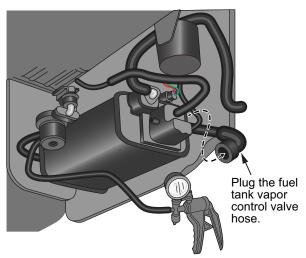
Watch the FTP sensor value on the HDS, and gently apply vacuum until the value reads approximately 2.10 V.
