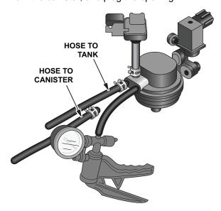
Watch the FTP sensor value on the HDS, apply vacuum until the value reads approximately
