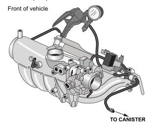
Enter the HDS PGM-FI menu, and select INSPECTION> EVAP TEST> MULTI SOLENOIDS. PCS ON> CVS ON> BPS ON.
