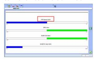
Apply vacuum to the system while monitoring the FTP sensor value reading on the HDS. Stop when the value reads approximately 1.50 V.
