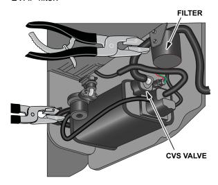
Enter the HDS PGM-FI menu, and select INSPECTION> EVAP TEST>MULTI SOLENOIDS> PCS ON> CVS ON> BPS ON.
