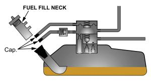
Watch the FTP sensor value on the HDS, and gently apply vacuum until the value reads approximately 2.10 V.
