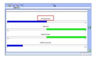
Apply vacuum to the system while monitoring the FTP sensor value on the HDS. Stop when the value reads approximately 1.50 V.
