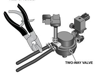
Pinch the hose between the CVS valve and EVAP filter.
