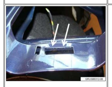
4. Before installing the taillight, inspect the trunk lid where the taillight was removed. Check the sheet metal area where the taillight hook is inserted. In this case, you can see by the reflection (white arrows) the sheet metal has been bent down by the hook during installation. This will not allow the hook to fully seat properly under the metal lip and needs to be corrected.
