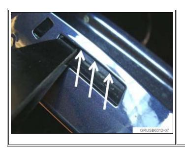
5. To correct this, insert a plastic tool as shown and gently pry up the inside metal lip in multiple steps for the entire length of the opening. The metal lip must be even and parallel to the opening for the hook to secure underneath the lip properly.
