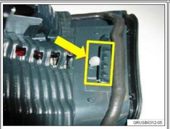
3. Clean the securing hook and metal trunk lid contact areas thoroughly; then apply the cold windshield adhesive to the center area of the securing hook, as shown. The adhesive application must be 4 to 5mm thick.
