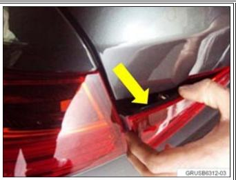
1. Check both rear trunk lid tail lamps for looseness or protrusion. If improper tail lamp fitment is noted, remove both left and right tail lamps. Refer to ISTA Repair Instruction 63 21 240 and 63 21 245.
