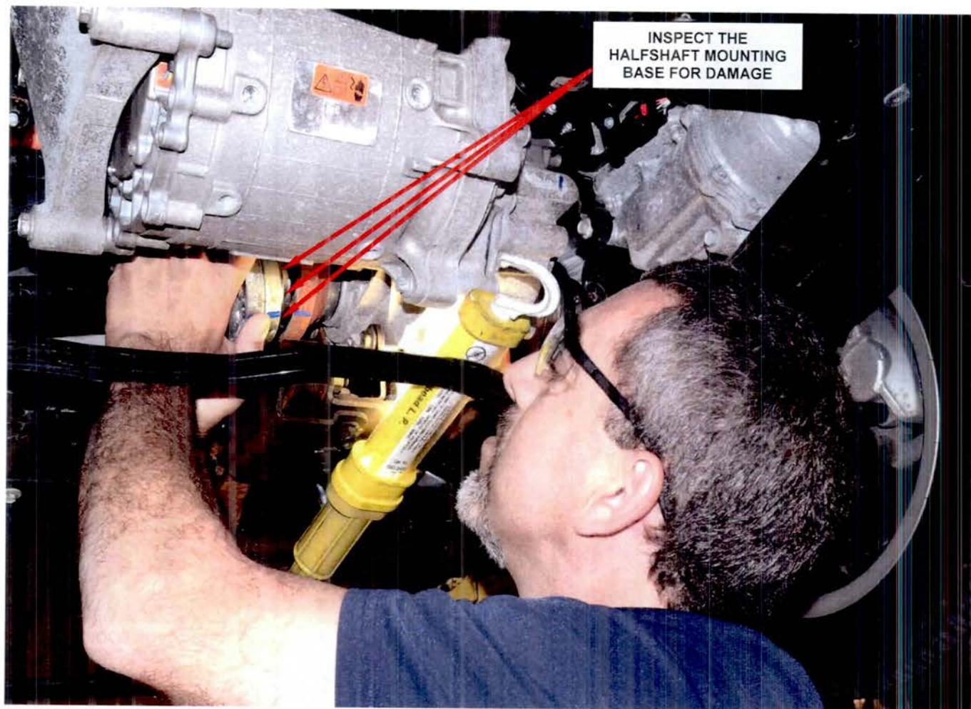
Figure 2 – Inspect the Halfshaft Base Mounting Surface (right side shown)
