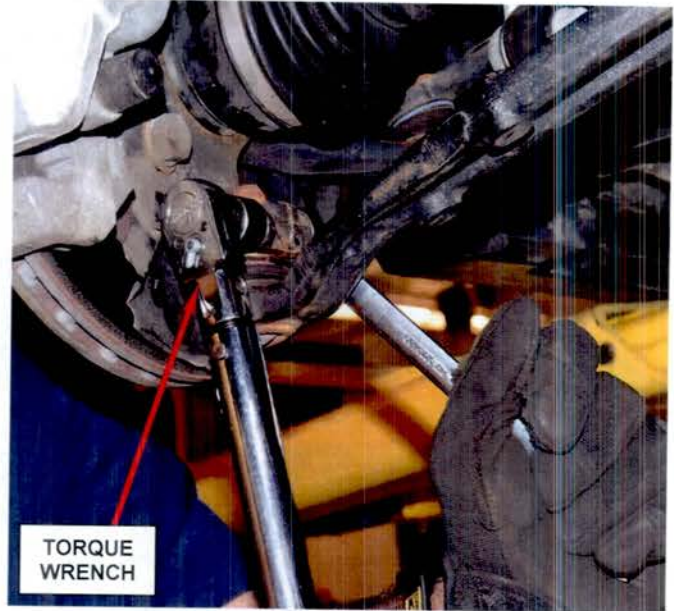
Figure 8 – Install New Pinch Bolt and Nut
