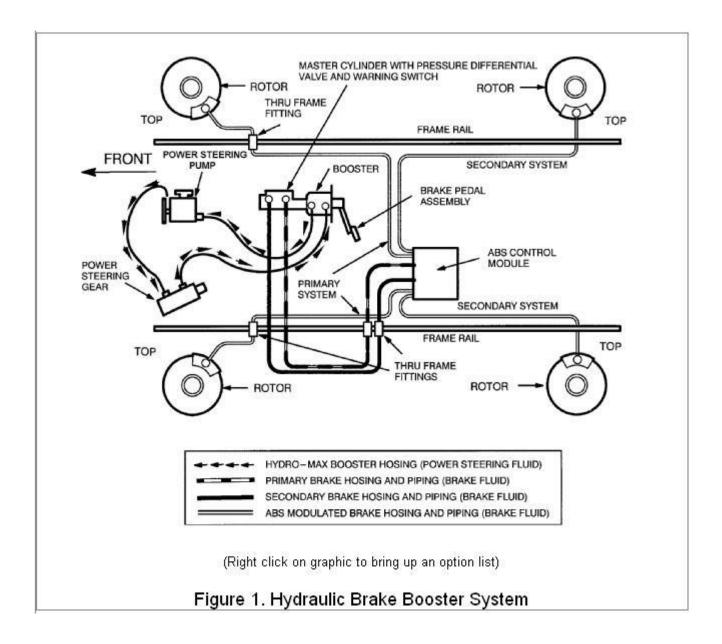
Referring to Figure 1, the hydraulic brake booster operates in series with the power steering gear. The power steering pump supplies the fluid flow and pressure demand to both units during steering and braking. When steering and braking action occurs simultaneously the pressure demand from the steering gear and brakes is additive.
