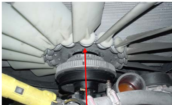
Fig. 6— Remove the engine cooling fan and lean it against the radiator.
