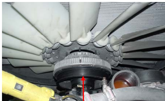
Fig. 7— Remove the fan drive assembly. Note: it will require an additional person to lift the fan drive out and under the vehicle.
