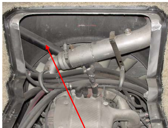
Fig. 5— Remove upper coolant tube .
