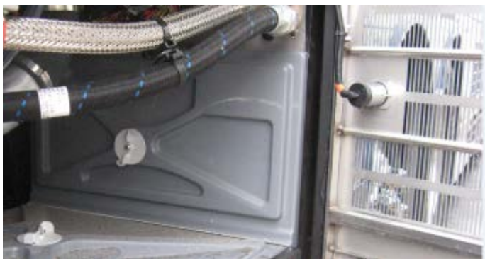
Fig. 2 Electrical compartment cover (X series vehicles)
