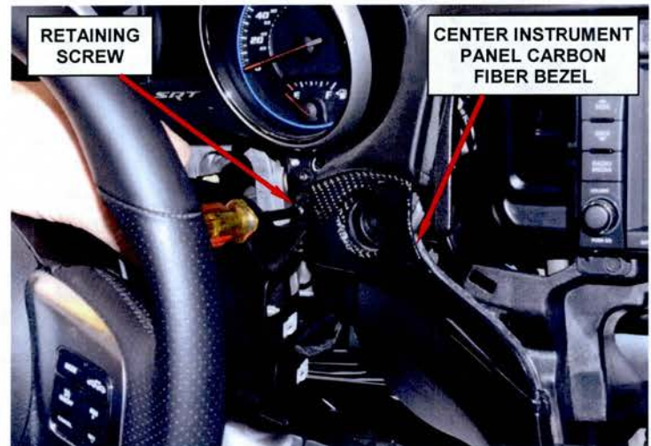
Figure 9 – Center Bezel Retaining Screw
