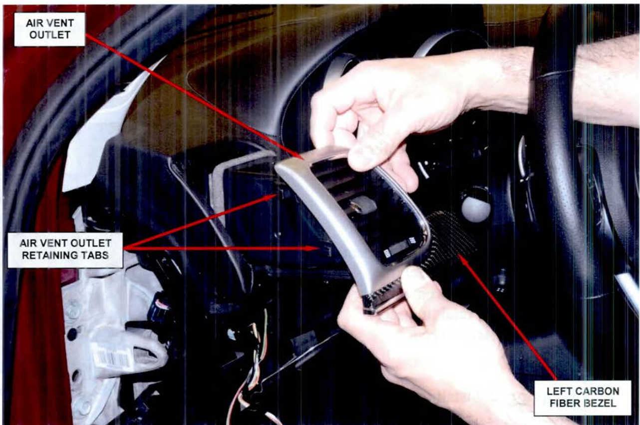
Figure 11 – Air Vent Outlet and Left Bezel Assembly
