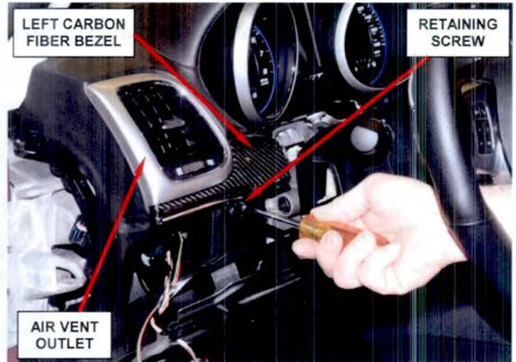
Figure 10 – Left Bezel Retaining Screw
