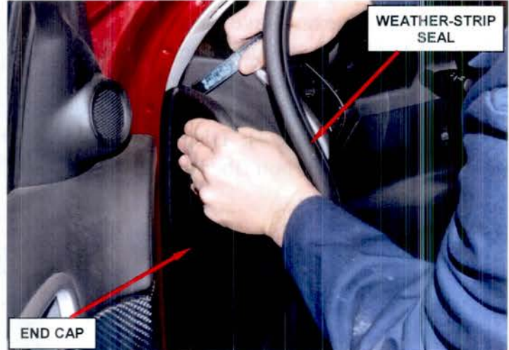
Figure 6 – Left Instrument Panel End Cap
