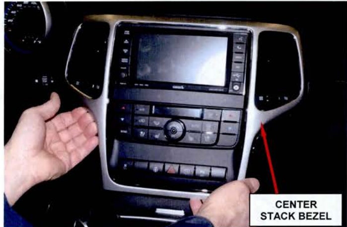
Figure 1 – Unsnap Center Stack Bezel
