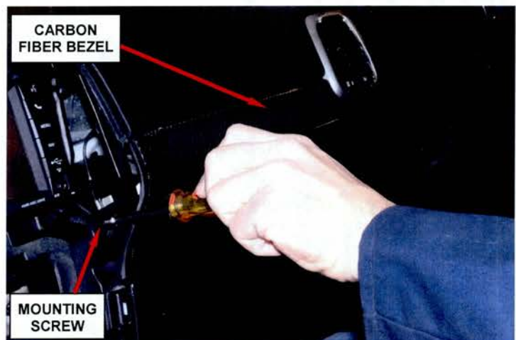
Figure 2 – Bezel Mounting Screw
